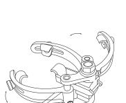
Two adjustable arms with hooks need to grab the spring firmly. The adjustable arms can go up and down and the hooks can slide sideways. Make sure to pull up the adjustable arms all the way up before pushing down the arm to grab the spring.
