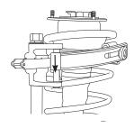
Make sure that the three hooks form a triangle with equal pressure on the spring. Turn the handle lever clockwise until the strut is loose. Unscrew the nut and replace the strut.
