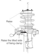
Slide in the middle hook and turn the handle lever clockwise to lower the gear down until the hook grabs the spring.
